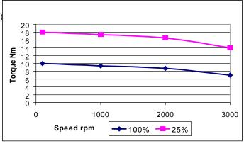
Data were measured on an HDD14J-Pa series motor mounted on a vertical 450 x 375 x 30 mm steel plate in free air, with a winding temperature rise of 90°C and driven by a commercially available inverter.
